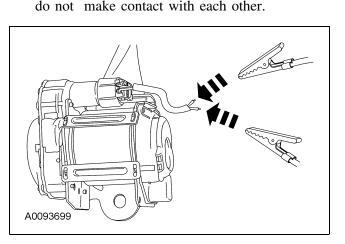
8. **NOTE:** Make sure to maintain the connections to the safety belt buckle or retractor.
