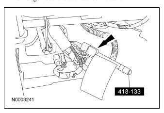
4. Connect the driver side air bag module electrical connector and reset the red locking tab.
