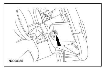
13. Install the 2 driver air bag module bolt caps in the steering wheel (1 shown).
