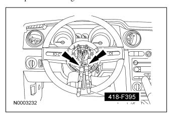
11. CAUTION: The clockspring electrical connectors are unique and cannot be reversed when connected to the driver air bag module. Match the electrical connector key to the keyway in the driver air bag module. Do not force the electrical connectors into the driver air bag module.
