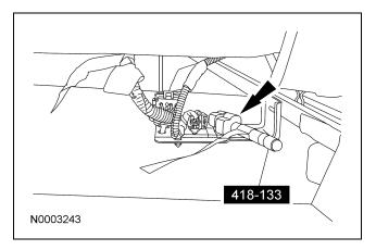
17. Release the red locking tab and disconnect the driver side air bag module electrical connector.
