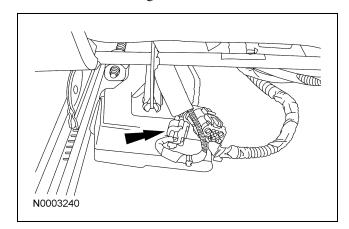
18. Attach the restraint system diagnostic tool to the vehicle harness side of the driver side air bag module electrical connector.
