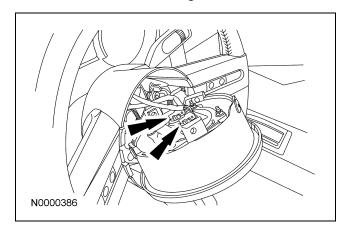
10. Attach the restraint system diagnostic tools to the clockspring electrical connectors at the top of the steering column.
