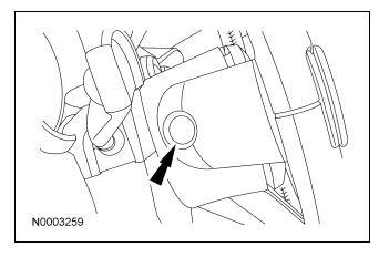
8. Remove the 2 driver air bag module bolts (1 shown).
