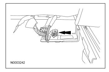
16. Attach the restraint system diagnostic tool to the vehicle harness side of the passenger side air bag module electrical connector.
