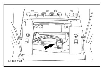
13. Attach the restraint system diagnostic tool to the vehicle harness side of the passenger air bag module electrical connector.
