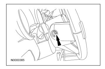
NOTE: Label the driver air bag module squib number on the driver air bag module electrical connectors before disconnecting.
