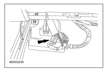
Remove the restraint system diagnostic tool from the vehicle harness side of the passenger side air bag module electrical connector.
