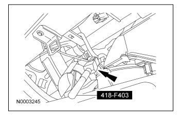
8. Connect the passenger air bag module electrical connector.
