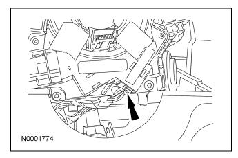
12. Remove the 4 clockspring screws and remove the clockspring.
