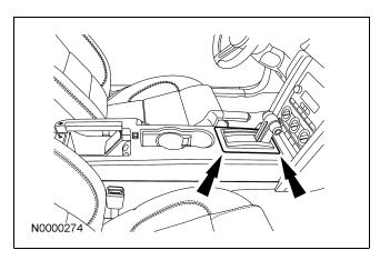
3. Remove the 2 screws and the center console top finish panel.
