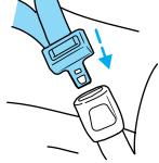
5. To put the retractor in the automatic locking mode, grasp the shoulder portion of the belt and pull downward until all of the belt is extracted and a click is heard.
