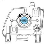
Handle a halogen headlamp bulb carefully and keep out of children's reach. Grasp the bulb only by its plastic base and do not touch the glass. The oil from your hand could cause the bulb to break the next time the headlamps are operated.
