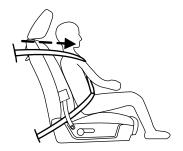
Allow the belt to retract. As the belt retracts, you will hear a clicking sound. This indicates the safety belt is now in the automatic locking mode.
